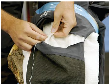
Figures 3a and 3b: The tech fibers stopped the chain on the third layer.
