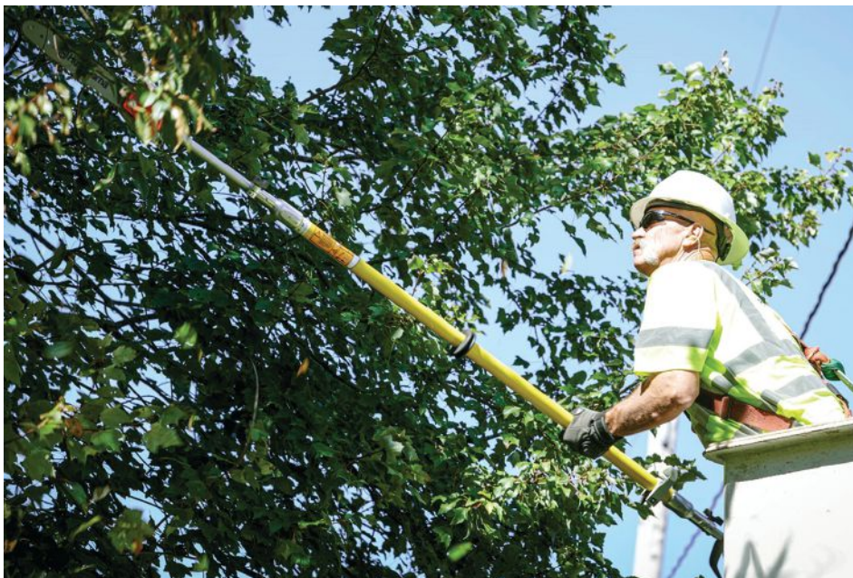
Husqvarna’s MADsaw (minimum approach distance saw), a dielectric pole pruner, made its debut in 2021. Photo courtesy of Husqvarna.
